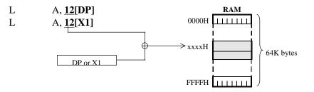
If an odd address is specified, then the data word starting at the even address immediately below it will be accessed ( $\rightarrow$ word boundary).
