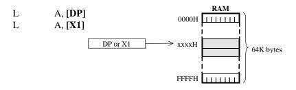
If an odd address is specified, then the data word starting at the even address immediately below it will be accessed ( $\rightarrow$ word boundary).
