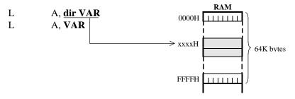
If an odd address is specified, then the data word starting at the even address immediately below it will be accessed ( $\rightarrow$ word boundary).
