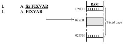
If an odd address is specified, then the data word starting at the even address immediately below it will be accessed ( $\rightarrow$ word boundary).
